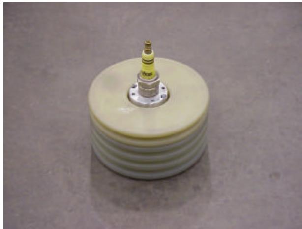
Figure 7. Schematic diagram and photograph of the triggered hydrogen switch designed for high repetition rate
