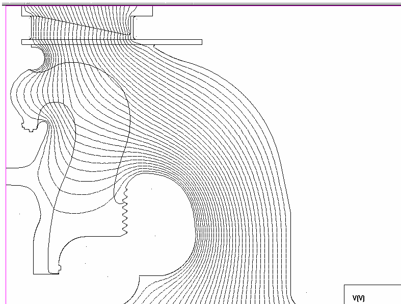
(b) JOLT transfer switch design in closed mode.
